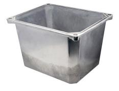
The ZA-8 alloy, composed primarily of zinc, aluminum, copper, and magnesium, offers a winning combination of strength, durability, and corrosion resistance. In the context of antenna mounts and enclosures, this alloy's tensile strength of approximately 42,000 psi ensures robust structural integrity. It is crucial in outdoor environments where exposure to varying weather conditions and mechanical stress is inevitable.
